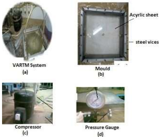
Figure-1: Locally developed VARTM system. (a) VARTM system, (b) Acrylic sheet mould, (c) Compressor (vacuum pump), and (d) Pressure gauge.
