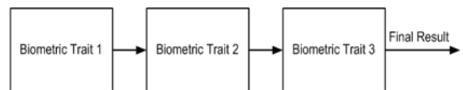
Figure 2: Serial arrangement of multi-modal biometric system
