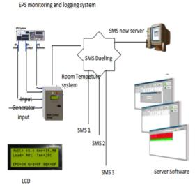
Fig. 3: Workflow for EPS monitoring and logging system.
